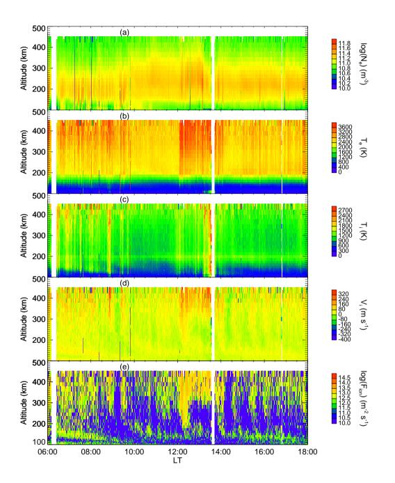
**Figure 2.** EISCAT Svalbard Radar (42 m dish) parameter plot for dayside 11 September, 2007. The panels a - e are respectively the electron density, electron temperature, ion temperature, ion drift velocity and the ion flux.
