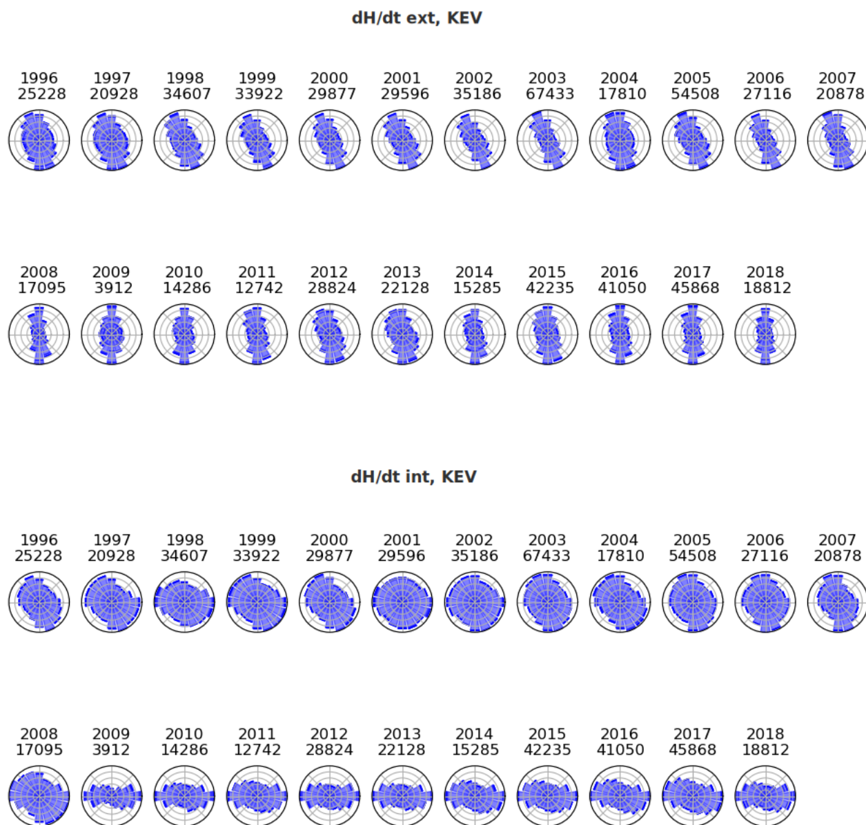
Figure A1. Yearly directional distributions of d\mathbf{H}/dt at Kevo (KEV), 1996-2008. Upper panel: external d\mathbf{H}/dt , lower panel: internal d\mathbf{H}/dt . The number of data points is plotted under the year label.
