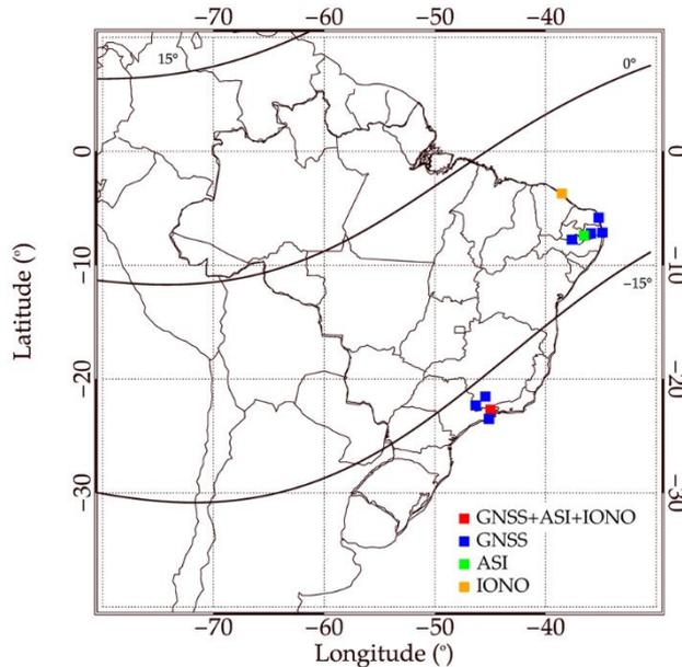
**Figure 1:** Map indicating the geographic locations of the instruments used in this study. The red symbol represents the site where GNSS receiver, All-Sky Imager (ASI), and ionosonde (IONO) are available. Blue symbols represent sites with only GNSS receivers, while green symbols indicate ASI sites, and orange symbols represent IONO sites. The black lines identify the magnetic equator (0 degrees) and low latitudes (near  $\pm 15$  degrees) for the year 2016.
