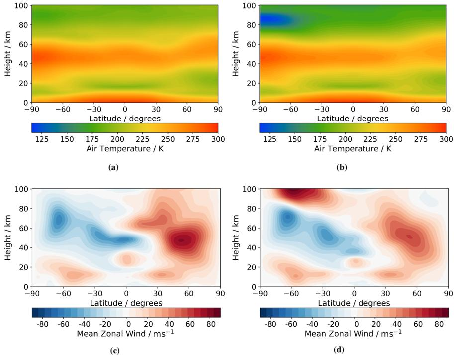
**Figure 1.** Latitude-height zonal-mean monthly-mean climatologies in December comparing (a) ExUM temperature before with (b) ExUM temperature after the non-LTE implementation. Also compared is (c) ExUM zonal ( $u$ ) wind before with (d) ExUM zonal ( $u$ ) wind after the non-LTE implementation. The more accurate modelling of the summertime polar mesopause minimum is evident upon introduction of the non-LTE radiation scheme with consequent effect on the modelled winds in the MLT.
