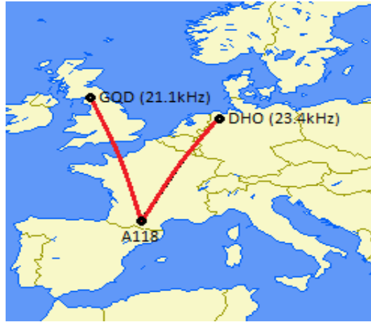
Figure 1. VLF signal propagation paths (DHO-A118 and GQD-A118) used in the study. Map adopted from A118 channel details at https://sidstation.loudet.org/channels-details-en.xhtml
