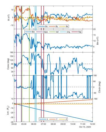
**Figure 3.** Magnetometer data in the magnetosheath and tail. From top to bottom: the three components of the magnetic field in VSO-coordinates; the magnitude of the magnetic field; the cone angle; the clock angle; and the location of the spacecraft in VSO-coordinates. The purple, green, blue and red dotted vertical lines show the intervals of interest.
