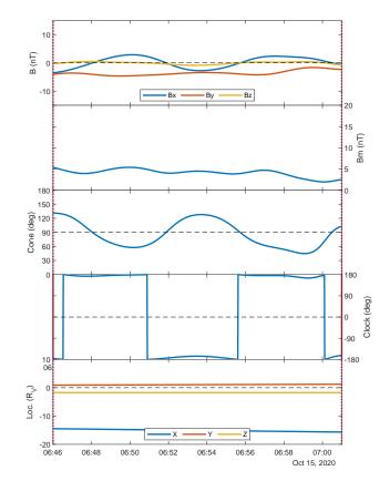
**Figure 7.** Zoom in on magnetotail flapping interval (red). The cone-angle clearly shows alternating magnetic field directions (tailward  $\theta_c > 90^\circ$  and Venusward  $\theta_c < 90^\circ$ ). The clock-angle remains basically the same ( $\phi_c = 180^\circ \equiv \phi_c = -180^\circ$ ).
