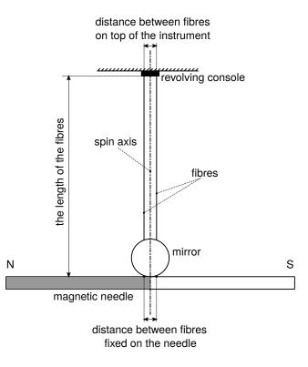
Figure 3. A sketch of the fibres, magnetic needle and mirror in the bifilar magnetometer.
