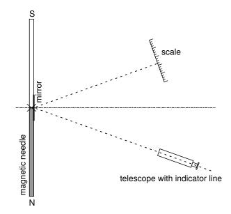
Figure 4. The top view of the bifilar magnetometer, mirror, telescope and scale.
