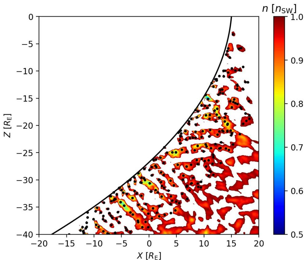
**Above: A plot showing ULF wave troughs / local minima as black dots within 10 RE from the bow shock at time t=900.0 s. The colormap shows values of proton number density below the input solar wind density  $n_{SW}$ . The bow shock is modelled with the 4th order polynomial described in the manuscript.**
