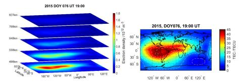
Figure 3: Subfigures top: Method Rotation reconstructed electron density represented by layers at different heights between 490 and 827 km (left) and vertical TEC map deduced from the reconstructed 3D electron density in the altitude range between 450 and 20200 km (right).
