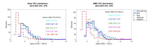
Figure 8: Plausibility check for the perturbed period – distributions of the delta TEC (left) and RMS (right) values.
