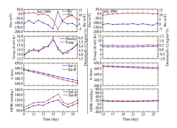
**Figure 11.** Corresponding mean daily variations in Dst, Bz,  $\rho$ , T, h and ODR for Sat-A and Sat-B during 09-20 July 2000 (left) and 15-26 July 2006 (right)
