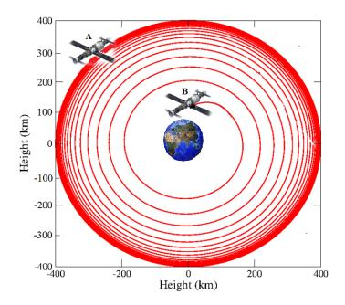
**Figure 1.** Orbital decay scenario of a LEO satellite due to atmospheric drag. The satellite orbit decreases from altitude "A" to altitude "B" as a consequence of atmospheric drag (Adapted from Nwankwo (2016)).
