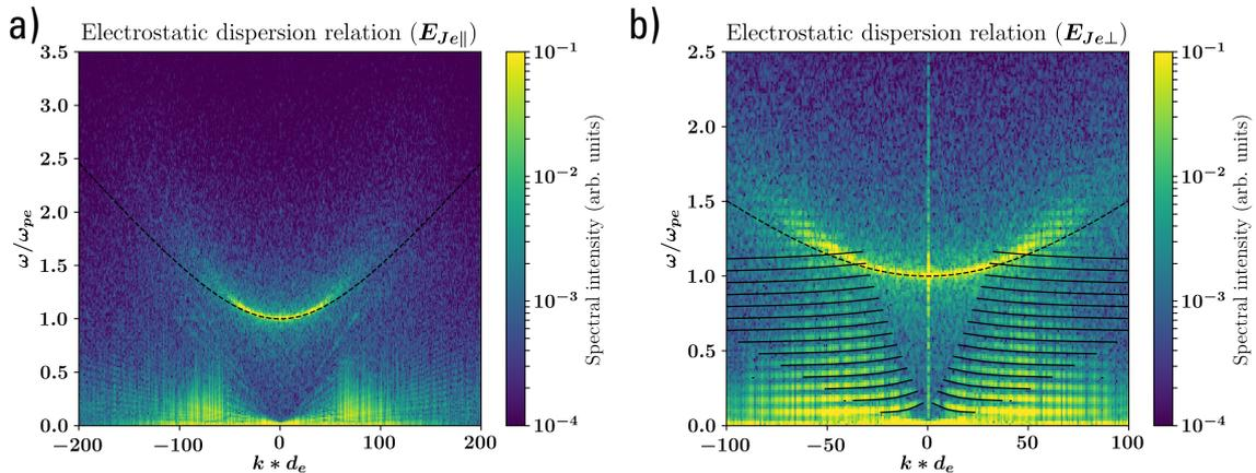
**Figure 4.** Dispersion analysis of the electron solver in a 1D test case with an axis-parallel (panel a) and axis-perpendicular (panel b) magnetic field. The colormap shows the spatiotemporal Fourier transform of  $E_{J_{e\parallel}}$  (panel a) and  $E_{J_{e\perp}}$  (panel b) overlaid with analytical solutions for the Langmuir wave (black dashed curve) and Bernstein modes (black solid curves).
