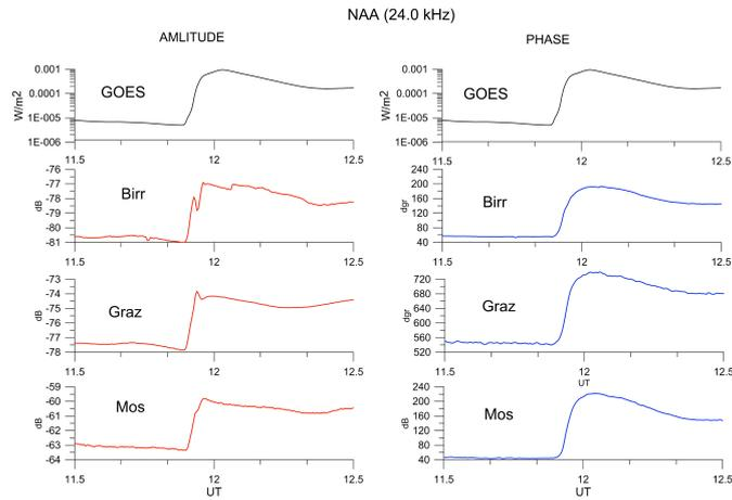
**Figure 2.** Amplitude (left) and phase (right) anomalies recorded in the NAA signal in Birr, Graz and Moscow receiving stations during the X-ray burst on September 6, 2017. Top panel shows X-ray flux measured with GOES satellite in the wavelength range of 0.05-0.4 nm.
