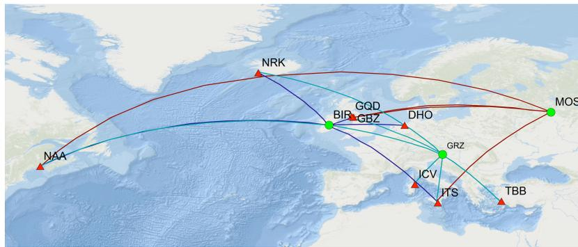
**Figure 1.** Positions of the receivers (green circles) in Birr, Ireland (BIR), Graz, Austria (GRZ) and Moscow, Russia (MOS) together with positions of the eight transmitters (red triangles), which have been used in this study.
