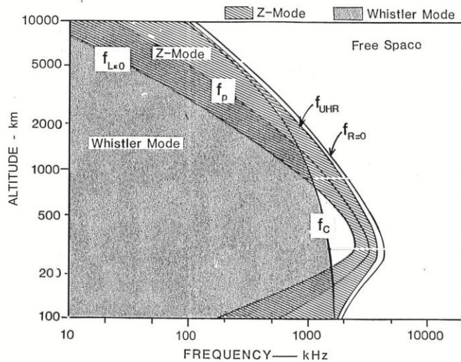
Thus, the observed waves by DEMETER are not free-space mode but R-X mode of whistler waves trapped in the plasmasphere. When the authors consider the LF wave propagation from the source region near the plasmapause to the low-altitude equatorial region, they should take into account the propagation characteristic of whistler mode waves with respect to the magnetic field.
