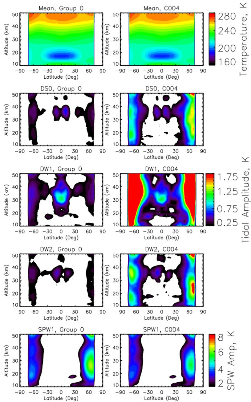
Fig 3. Annual means of mean temperature ( $T_0$ ) and amplitudes of diurnal tides (DS0, DW1, DW2) and stationary planetary wave (SPW1) for group G0 and satellite C004 during 2010 (Jan to Dec). Note the overestimation of amplitudes of the migrating tide, particularly in mid and high latitudes in the analysis of data over  $\pm 30$  days using a single satellite (C004).
