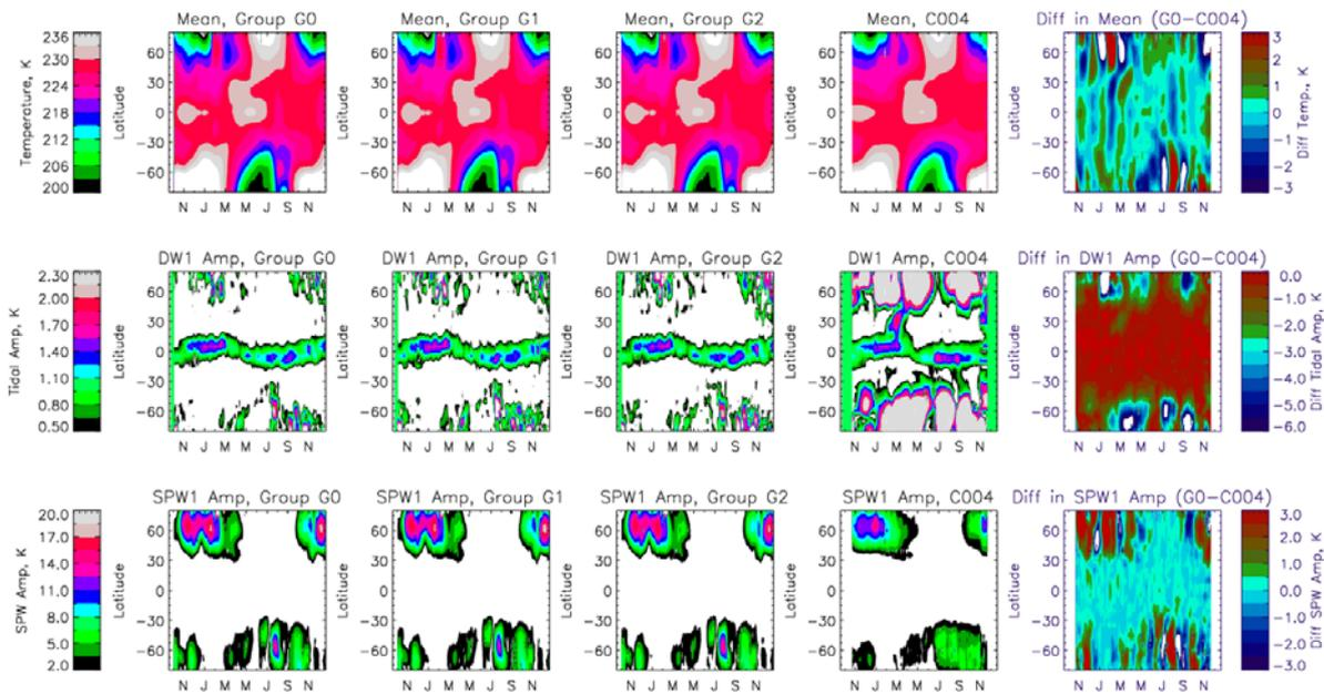
370 Fig. 2. Rows show the variation in mean temperature, amplitudes of the DW1 tide and SPW1 wave, respectively. Columns are results from groups G0, G1, and G2, and from satellite C004, respectively, for 30 km altitude. The last column is the numerical difference in results obtained from group G0 ( $\pm 10$  days' data) and C004 ( $\pm 30$  days' data).
