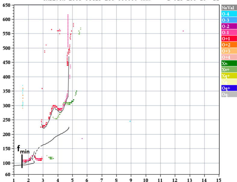
Figure 1. A typical daytime ionogram recorded at Chilton at 09:00 [UTC] on 15 October 2003 with the used fmin parameter marked. (Source of the ionogram is the GIRO network: Global Ionospheric Radio Observatory (GIRO, http://giro.uml.edu ))
