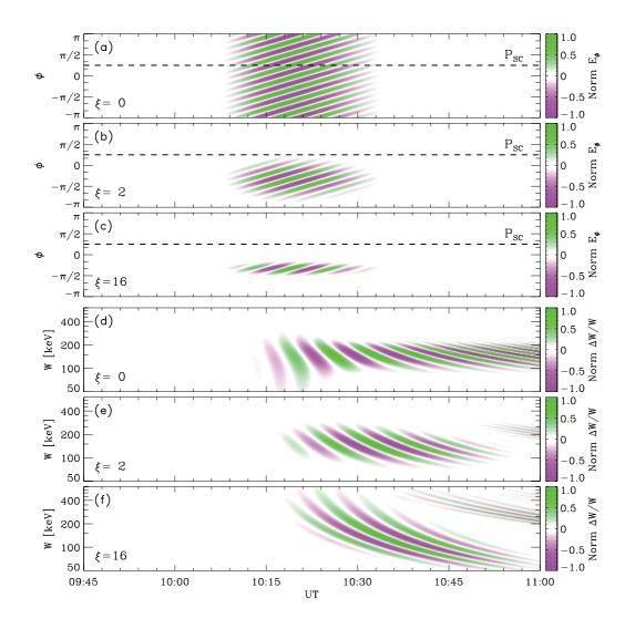
Figure 5. The width of electron flux modulation varied with the azimuthal distribution of the modeled ULF waves. (a)-(c) Modeled ULF waves of different spatial extents in the azimuthal direction. (d)-(f) The normalized electron energy gains from the corresponding ULF waves.
