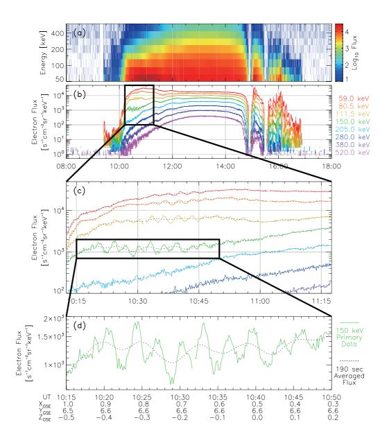
Figure 1. Overview of the electron flux observed by BD-IES. (a)(b) Spectrogram and series plot of the electron flux in a full pass of the spacecraft through the radiation belt on October 13, 2015. (c) Zoomed-in view of the electron flux oscillation. (d) Zoomed-in view of the multi-period electron flux modulation.
