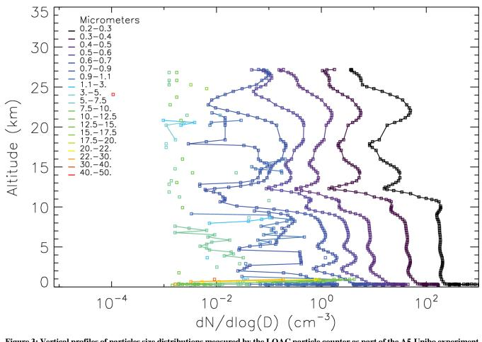
Figure 3: Vertical profiles of particles size distributions measured by the LOAC particle counter as part of the A5-Unibo experiment on the BEXUS18 stratospheric flight.
