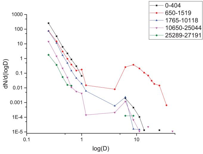
Figure 4: Average size distribution of aerosol particles as a function of height during BEXUS18 stratospheric flight. The five curves are obtained averaging the aerosol number densities as a function of the atmospheric layers pointed out by the temperature profile as follows: 1: 0-404 m (black line); 2: 650-1519 m (red line); 3: 1765-10118 m (blue line); 4: 10650-25044 m (pink line); 5: 25289-27191 m (green line).
