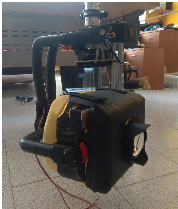
507 508 Figure 1. The 3-axis motorized gimbal stabilized platform, holding the NLC camera, 509 designed and built by the Aerospace laboratory "Stratonautica". Photo by Denis Efremov.
