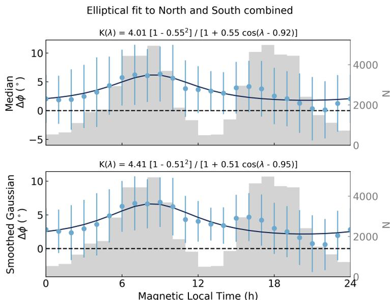
**Figure 3.** Elliptical boundary correction (black line) fit to the median (top) and S.G. peak (bottom)  $\Delta\phi$  for both hemispheres. The blue dots and scatter bars show the central value and  $\epsilon$  in each MLT bin. The grey histogram shows  $N_{MLT}$ , and scales to the y-axis on the right.
