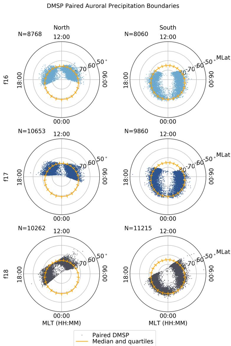
**Figure 1.** Paired AMPERE R1/R2 boundaries and DMSP SSJ OCBs for both hemispheres (northern in the left column and southern in the right column) and each satellite. The scattered points show the DMSP SSJ OCBs, while the gold circle shows the median location of the AMPERE R1/R2 boundaries. The scatter bars denote the quartiles of the paired AMPERE R1/R2 boundaries.
