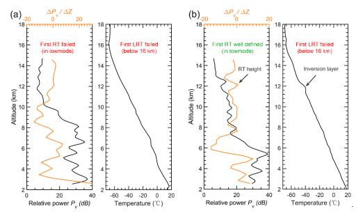
**Figure 12.** Example profiles of radar echo power and radiosonde temperature that (a) both the RT and LRT definitions fail due to the continuing decrease in temperature on 00 UTC 7 July 2012 and (b) the temperature inversion layer failed to meet the LRT definition but well defined in RT definition on 12 UTC 02 August 2012. Please note that we only consider the conditions below 16 km.
