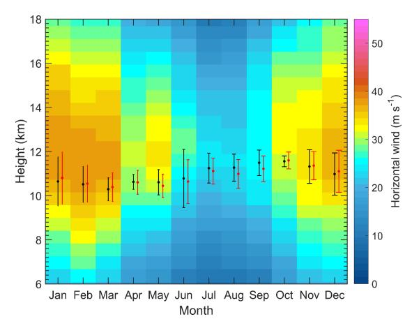
**Figure 9.** Height-time intensity map of monthly mean horizontal wind speed (shaded, m/s) derived from the middle mode of Beijing MST radar, during November 2011-May 2017. Also shown is the monthly mean height of RT (black dots) and LRT (red dots, offset by +6 days) along with the vertical error bars representing the standard deviations.
