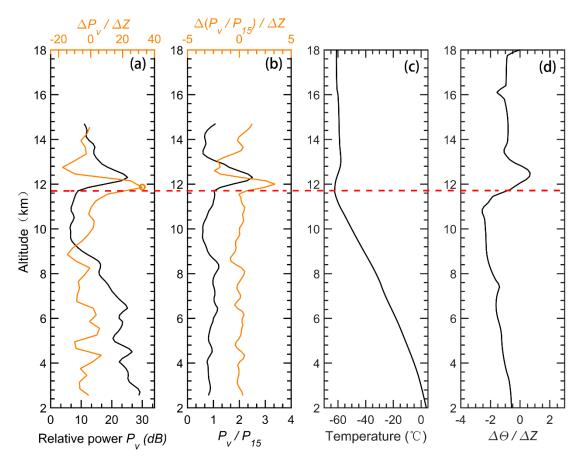
**Figure 2.** Example vertical profiles of (a) relative radar echo power (black line) along with its gradient variation (orange line), (b) radar aspect sensitivity (black line) along with its gradient variation (orange line), (c) radiosonde temperature and (d) potential temperature gradient on 00 UT 04 November 2011. The horizontal red dashed line marks the LRT height. The orange circle in Fig. 2a denotes the RT height.
