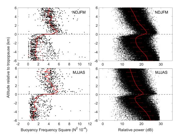
**Figure 7.** Scatterplots of (left panels) static stability (N<sup>2</sup>) and (right panels) radar relative echo power as a function of altitude relative to the LRT (left panels) and RT (right panels) for extended winter (NDJFM) and summer (MJJAS) seasons for two specific years 2012-2013. Red lines in each panel denote the corresponding mean profiles and the error bars indicate the standard deviations.
