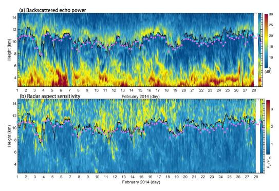
**Figure 3.** Altitude-time intensity plot of (a) radar backscattered echo power and (b) radar aspect sensitivity for February 2014. The tropopauses determined based on the radar echo definition are shown as a black solid curve. The cyan asterisks '\*' and pink dots indicate the location of the LRT derived from simultaneous twice daily radiosonde data and the PVT from ECMWF ERA-Interim reanalysis, respectively. White stripe indicates the time frame of radar missing data.
