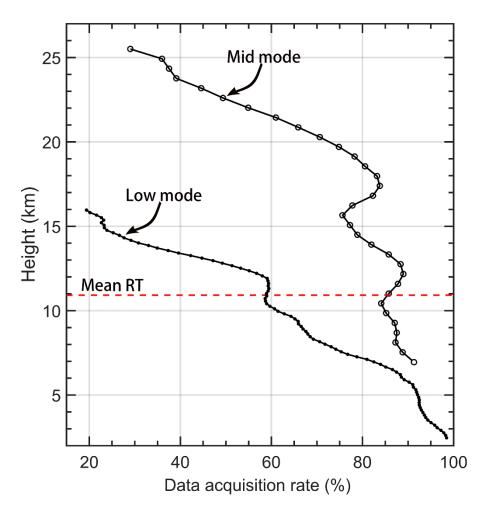
**Figure 8.** Vertical height profiles of the averaged effective radar wind data acquisition rate in low mode and middle mode during November 2011-May 2017. The red dashed line indicates the mean RT height.
