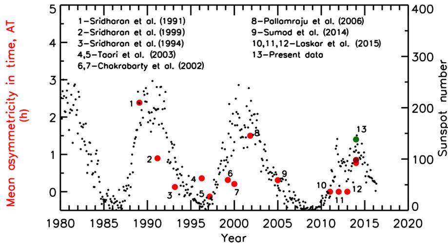
**Figure 8.** Variation of mean asymmetry in time (AT) at OI 630.0 nm emissions in different years as obtained from the published literature is shown. The monthly averaged sunspot number is also plotted. A striking similarity between them indicates that the equatorial electric field has a direct role in the observed diurnal behaviour of the neutral optical dayglow emission intensities.
