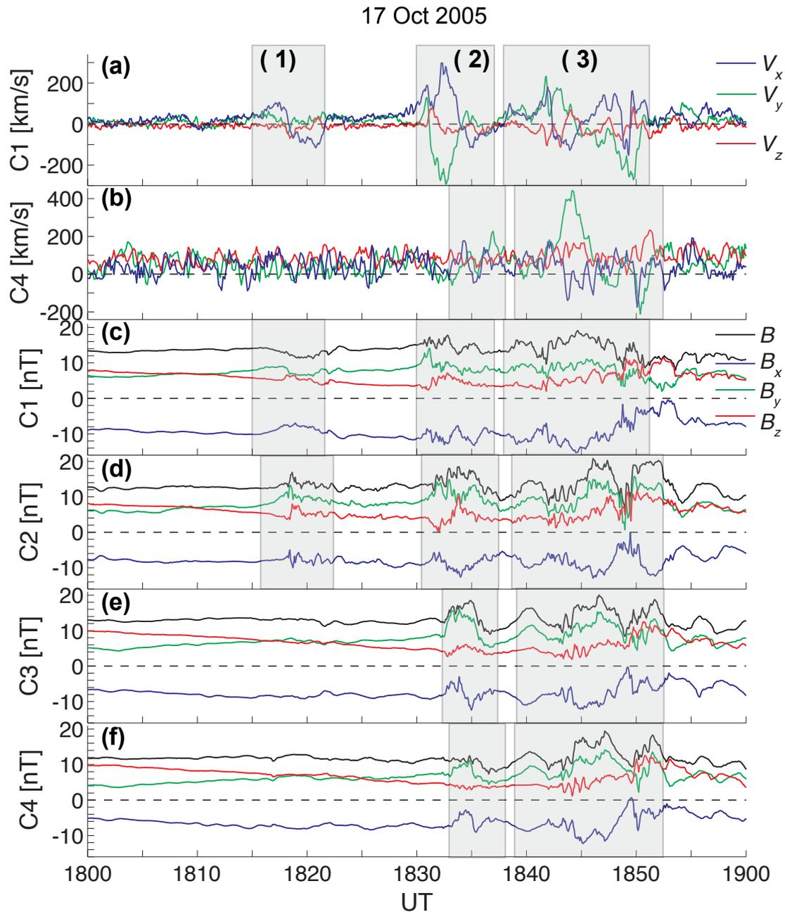
**Fig. 4.** Cluster data on 17 October 2005. (a) C1 CIS HIA velocity components in GSM. (b) C4 CIS CODIF proton velocity components in GSM. (c)–(f) Spin resolution magnetic field components by FGM in GSM. The vertical grey-shaded strips indicate the flow events under study.
