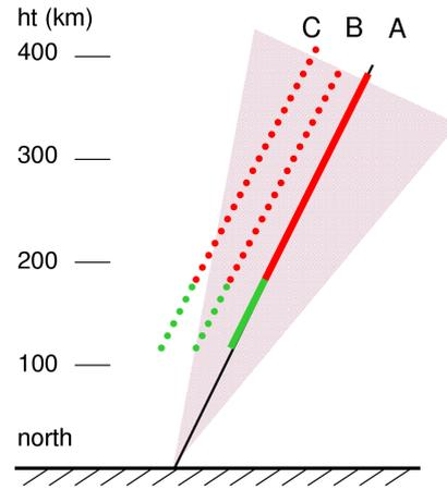
**Fig. 12.** Schematic diagram (not to scale) of the geometry of the HiTIES spectrograph with auroral arcs in three positions in the field of view. The shaded area represents the 8° slit along the magnetic meridian. Arc at position A corresponds to the magnetic zenith.
