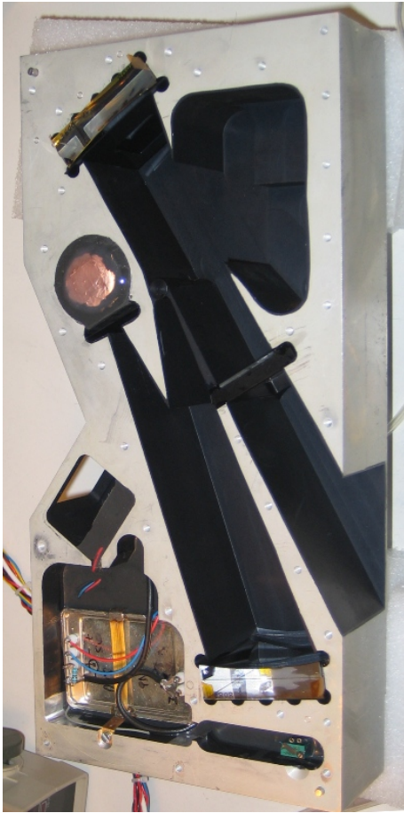
Fig. 9. The open SLAM instrument (without the cover plate) complete with gratings, photomultiplier tube, and electronics, the entrance is to the right and an additional sun sensor is to the left.
