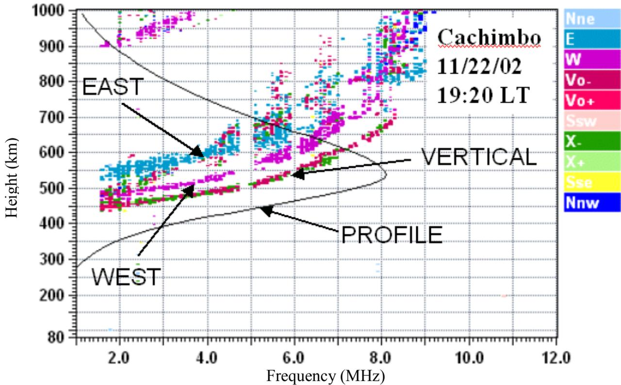
**Fig. 3.** Multi-directional ionogram at Cachimbo for 22 November at 19:20 LT showing echo traces from the west, east, and overhead, with an overlay of the vertical electron density (plasma frequency) profile.
