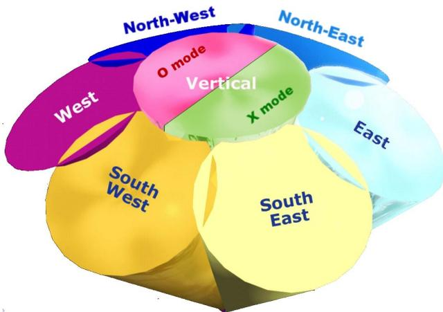
**Fig. 6.** Seven digitally synthesized beams for ionograms measurements.
