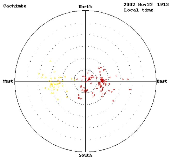
**Fig. 4.** Cachimbo skymap for 22 November at 19:13 LT showing echoes from the west with Doppler frequencies of -0.5 Hz, and from the east with Doppler frequencies of -2.0 Hz. The skymap displays zenith angles from 0 to 20°.
